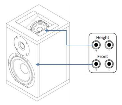
Figure 3: Integrated Dolby Atmos enabled speakers include both traditional speakers and upward-firing speakers in the same cabinet. The two sets of speakers have individual posts.
