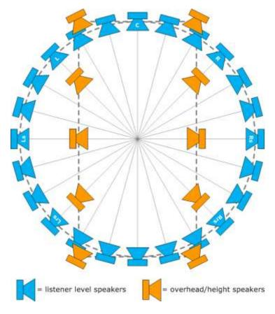
Figure 10: Dolby Atmos for home theaters supports as many as 24 speakers on the floor and 10 speakers producing overhead sound.
