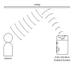
Figure 2: Dolby Atmos enabled speakers reflect sound off the ceiling to produce an incredibly lifelike re-creation of overhead sound.
