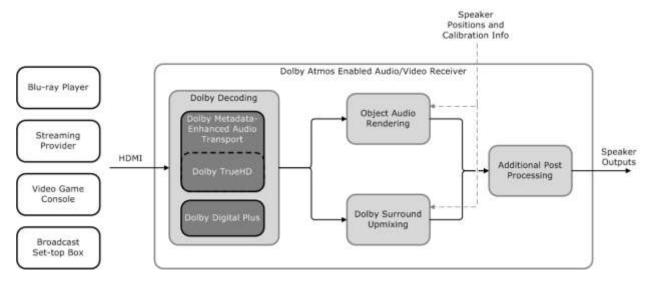
Figure 9: This diagram represents the workflow for translating cinematic Dolby Atmos content to home theaters.
